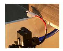
**CHECK SIDES** Ensure you have removed the hose and retaining knob from both sides of the pump.
