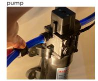
**REMOVE PUMP** Using a phillips screw driver remove all 4 screws and gently pull the water pump out.
