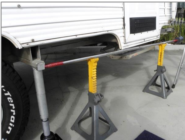
FIG. 4 HEAD CAP ENGAGEMENT TEST SET UP WITH TRAILER-MATE ADAPTER
