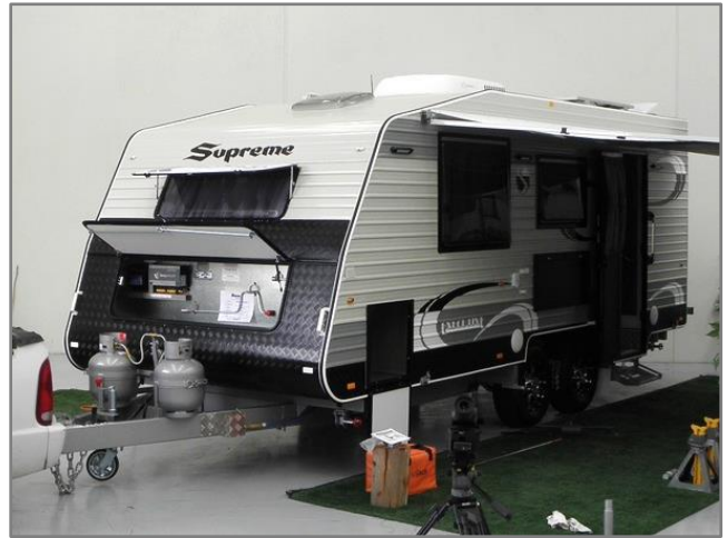
FIG. 3 'EXECUTIVE' CARAVAN WITH JACKING POINTS FOR BALL ADAPTER
