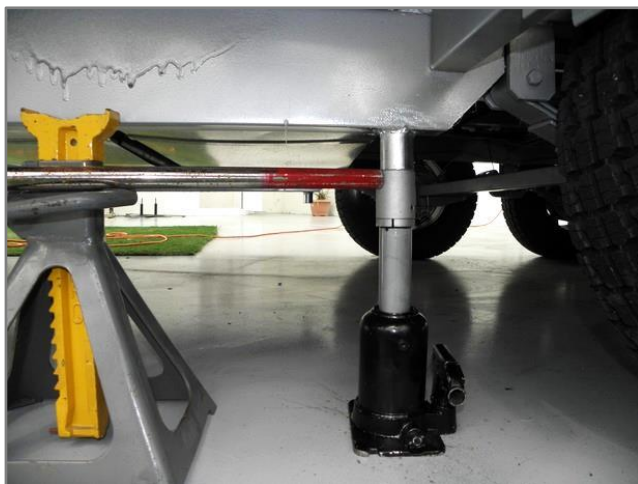
FIG. 6 HEAD CAP ENGAGEMENT TEST SET UP WITH BALL ADAPTER
