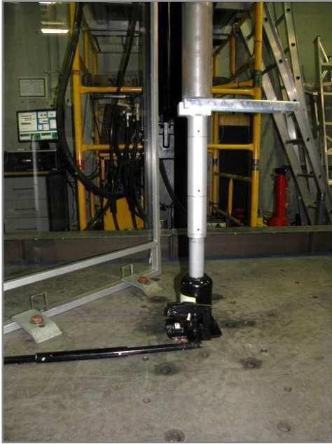
FIG. 8 OVERLOAD CAPACITY TEST WITH TRAILER-MATE ADAPTER
