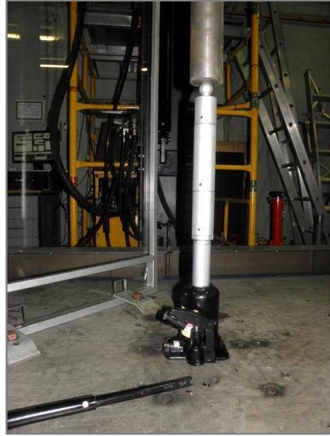
FIG. 9 OVERLOAD CAPACITY TEST WITH BALL ADAPTER
