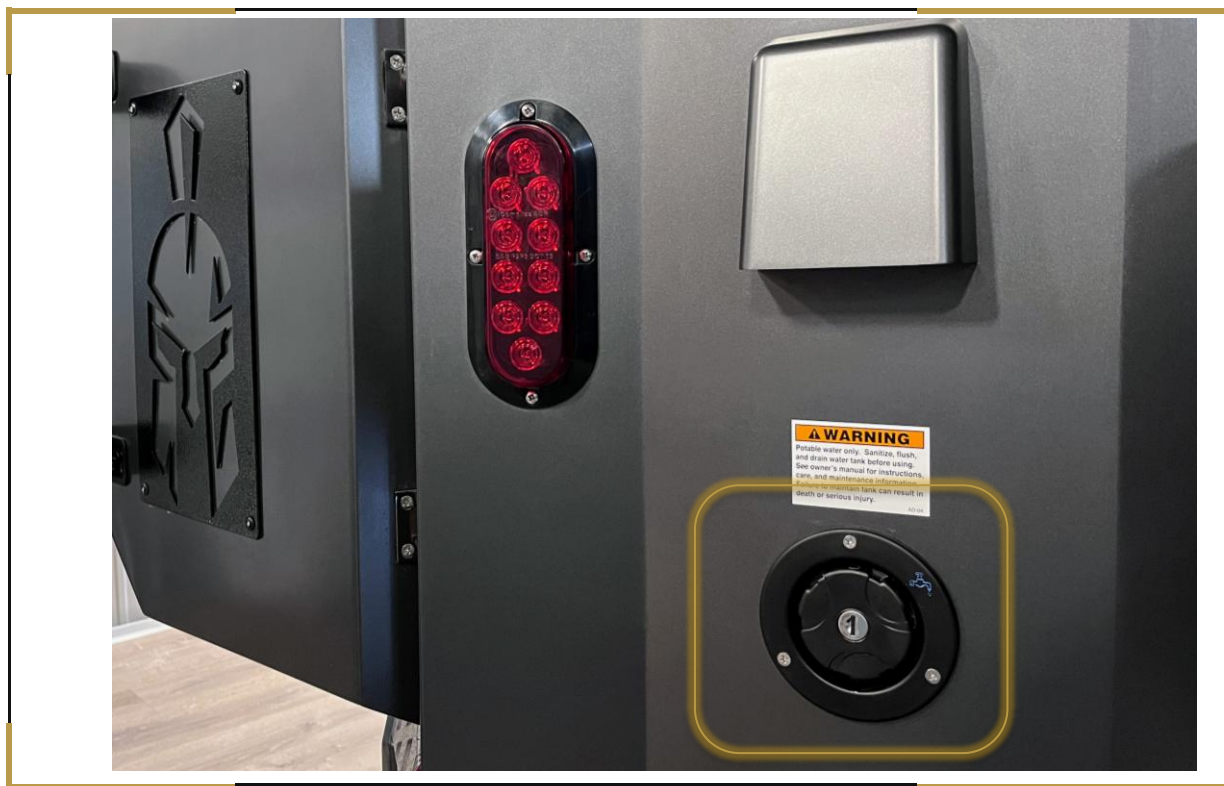
WATER FILL POINT LOCATION ON REAR OF CAMPER
