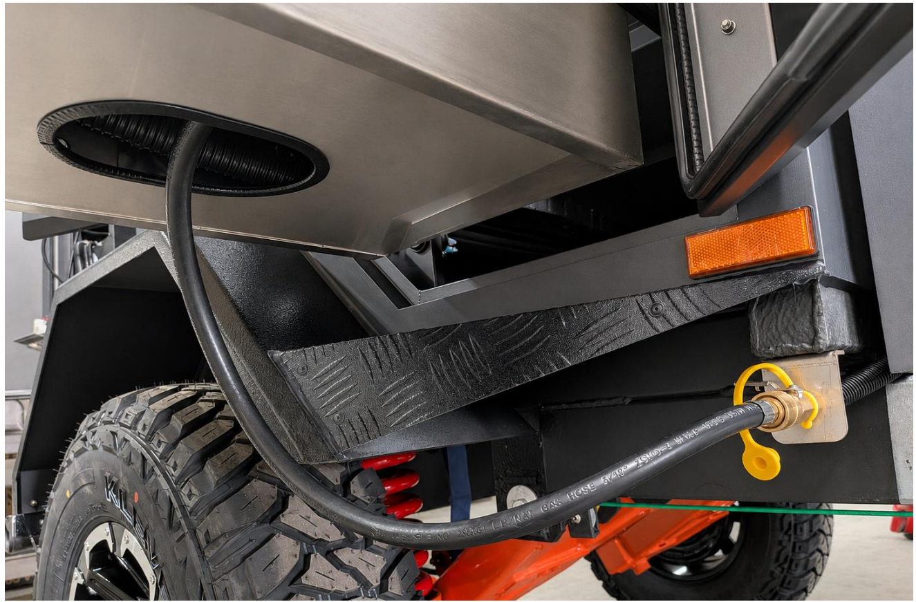
KITCHEN GAS HOSE CONNECTION POINT
